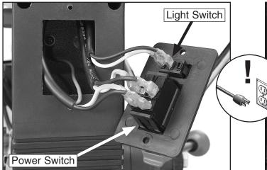
Figure 44. Power and light switch assembly.
